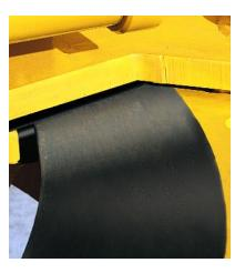
Duramide™ bearing material eliminates metal-to-metal contact and reduces the need for circle turn lubrication and adjustment. As well as being simple and cost-effective to replace, it has a minimum service life of more than 5,000 hours.
