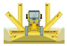
The MBCS gives you the flexibility to position the blade at any angle you need for shouldering, slope work and ditch cleaning – up to 90° upward and 21° downward.
