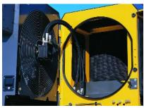
Since the grader's need for cooling depends on ambient conditions as well as the engine's power output, the variable-speed hydraulically driven fan on Volvo graders is designed to respond to actual demand. Combined with non-stacked coolers, the system continuously delivers just the right amount of cooling effort, consuming less fuel, producing less noise and maximizing available power for other grader functions.
