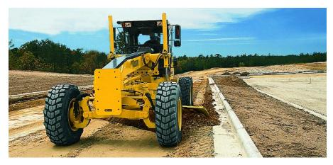
Whatever your application, the Volvo All Wheel Drive System is tuned to the task. The system provides an even distribution of power through independent variable displacement pumps and high torque motors at each front wheel. If the traction differs on either side, this system ensures that optimum pulling power is still achieved.
